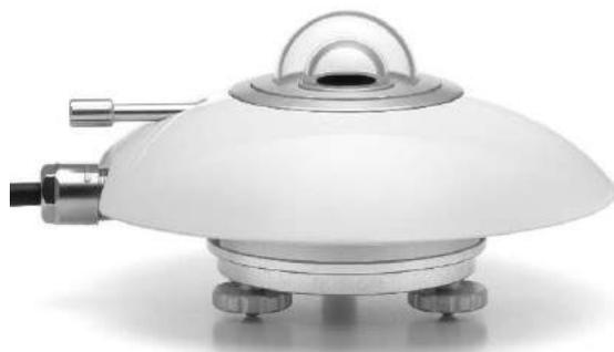
**Measured** hemispherical solar radiation
