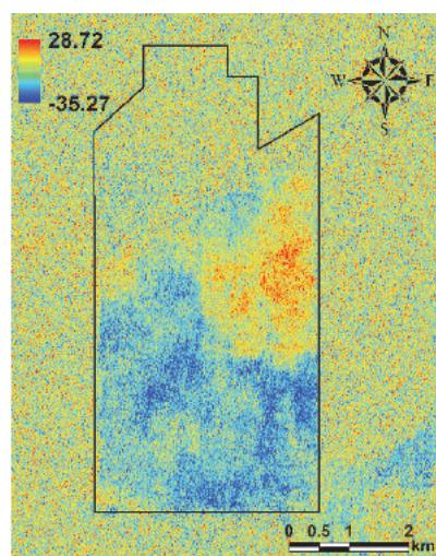
Figure 2. The distribution of total ground displacement (cm). Blue indicates subsidence, red means uplift, and the target region is in black.
