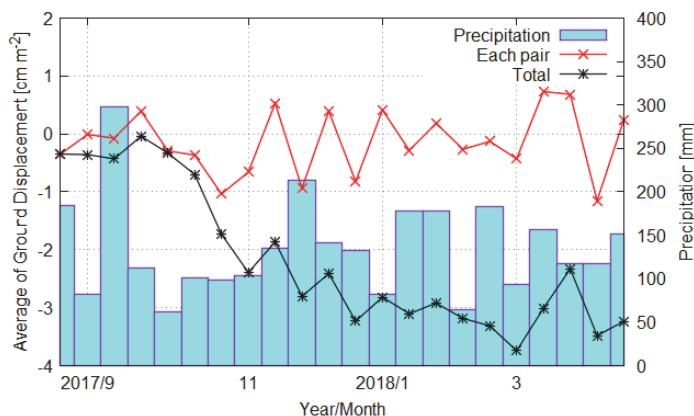
Figure 1. Ground displacement by InSAR processing. Red line is displacement every two time-series. Black-line indicates total displacement, and light blue bars are precipitation.
