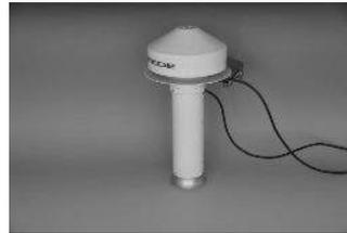
The PHF-02 is a sensor measuring the heat flux from a Wall or window. Especially. This is Epoxy resin. The sensor calibrate it individually and the pass heat capacity of the unit area output in mV.
