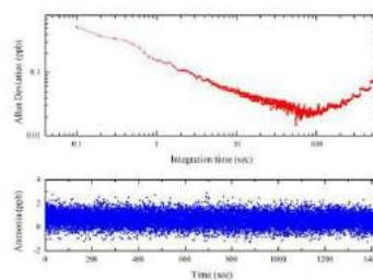
Fig. 2. An Allan deviation plot showing stability and precision of the  $\text{NH}_3$  sensor.
