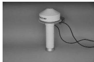
The PHF-02 is a sensor measuring the heat flux from a Wall or window. Especially. This is Epoxy resin.
