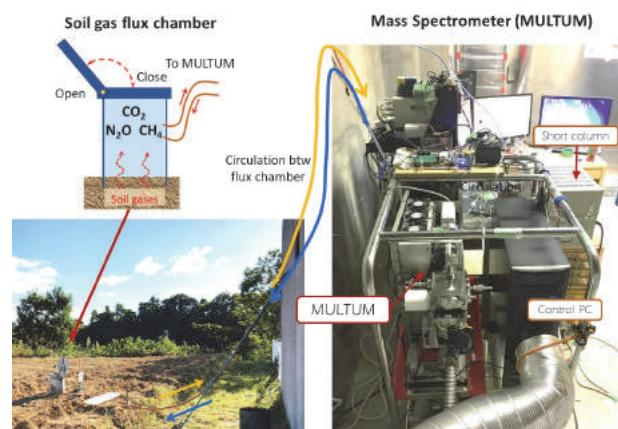
Figure 1. Schematic view of field observation in a soybean field at Ehime University farm. (Left) an automatic soil chamber, (Right) MULTUM mass spectrometer system.
